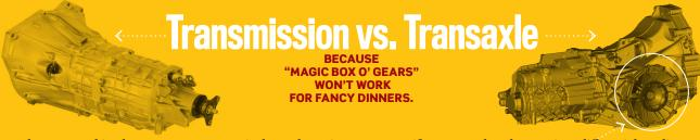
General term. Found in almost every car, even a single-speed EV. Sits somewhere between the power source and wheels, reducing or multiplying torque. Sometimes you shift it, sometimes it shifts itself. Aliases: gearbox (if it has gears and isn't a CVT), tranny.
