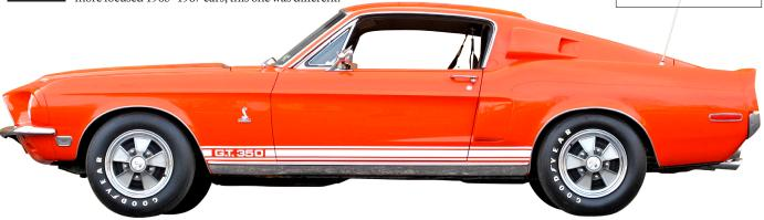
PARTS >> Original '68 Shelby parts are scarce and spendy. Fiberglass panels—nose, hood, trunk—are unique; most have been damaged. Repros can be spotted by a trained eye and hurt value. The hubcaps are 1968-only and run \$2000 for a restored set. Other valuable bits: shoulder harnesses and Lucas fog lamps.
